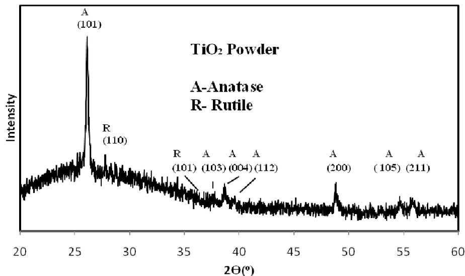
Figure 2 XRD pattern of TiO<sub>2</sub> powder.
