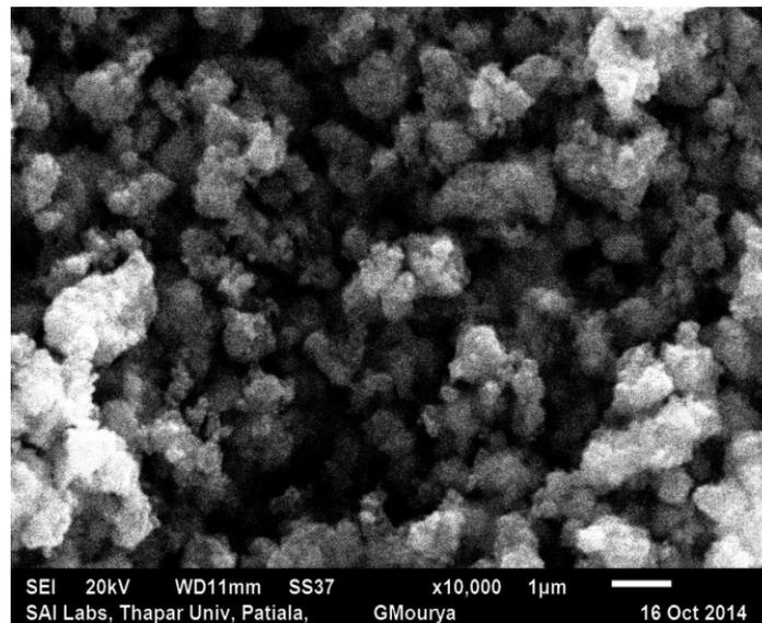
**Figure 4** SEM image of  $\text{TiO}_2$  Powder.
