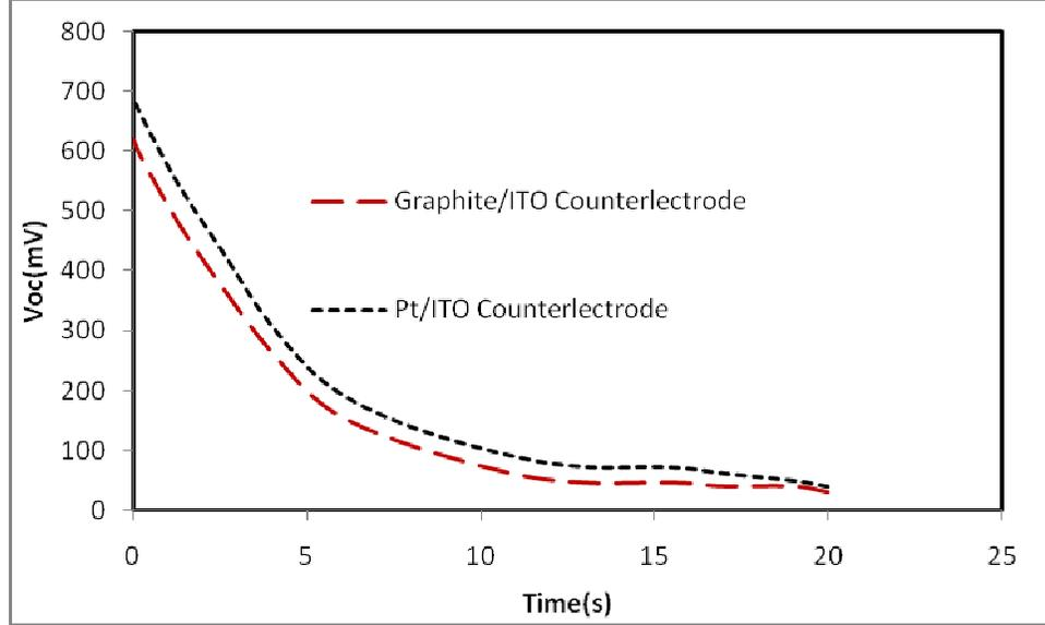
**Figure 11** Open circuit voltage decay with time.
