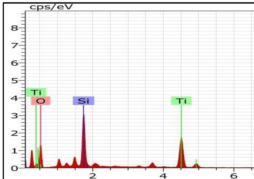
**Figure 6** EDX spectra of TiO<sub>2</sub> film.
