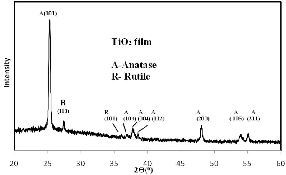
**Figure 3** XRD pattern of  $\text{TiO}_2$  film.
