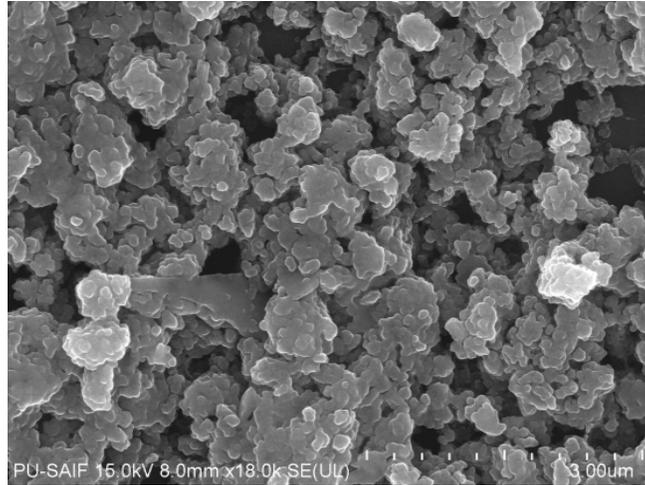
**Figure 5** FE-SEM image of TiO<sub>2</sub> film.
