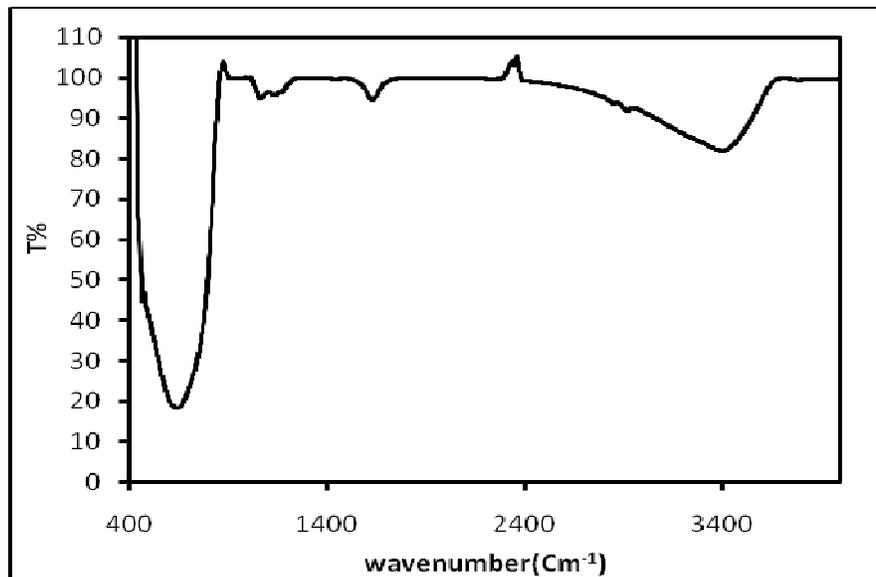
**Figure 7** FTIR of TiO<sub>2</sub> powder
