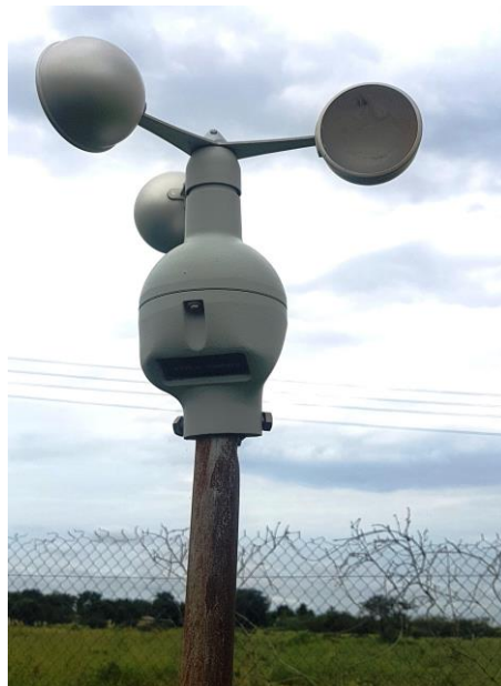
Figure 1: Cup Anemometer at Desert Research Center, Yobe State University
