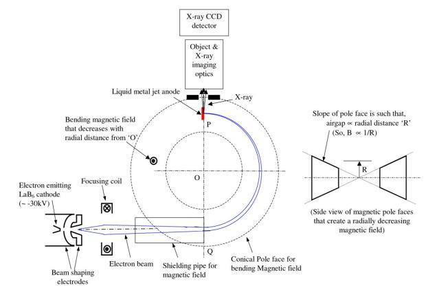
Figure 2. Schematic of the proposed high power microfocus X-ray source using a bent electron beam.
