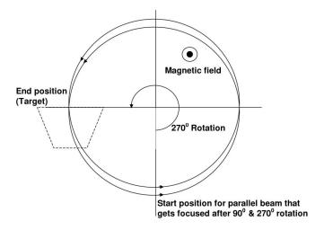
**Figure 1.** Focusing along one dimension by geometrical crossover in conventional transverse type electron guns
