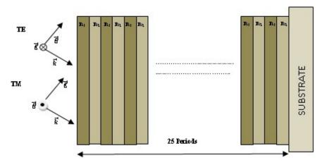
Figure 2: Schematic representation of proposed structure (AB)<sup>25</sup> with all A's as Cryolite and all B's as Ge
