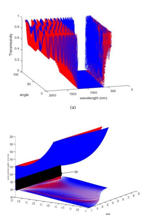
Figure 4: (a) Transmissivity variation with wavelength and angle of incidence (deg.) for TE modes (Red lines) and TM modes (Blue lines) in multilayered Cryolite-Ge.
