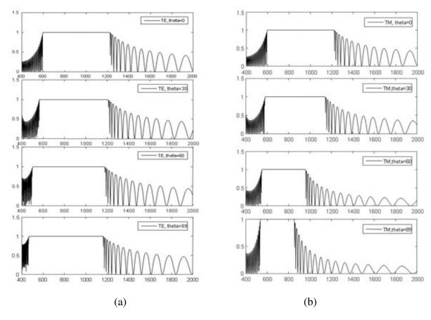
Figure 3. The reflectance spectra for TE and TM modes showing the total reflection region and bandwidth for  $n_1=1.34$ ,  $n_2=4.2$ ,  $d_1=149.25$  nm,  $d_2=47.61$  nm and N=25 at various incident angles,
