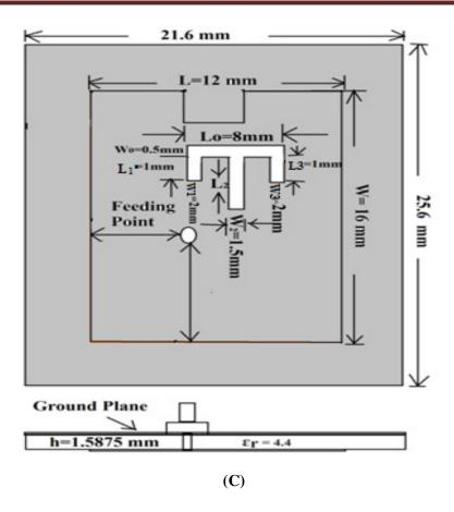
Figure 1 Geometry of the proposed antenna:
