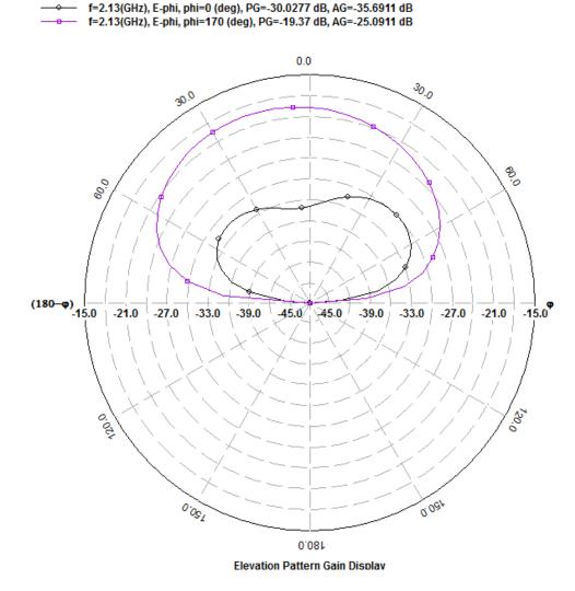
Fig. 3.9(b) Proposed antenna H- Plane pattern
