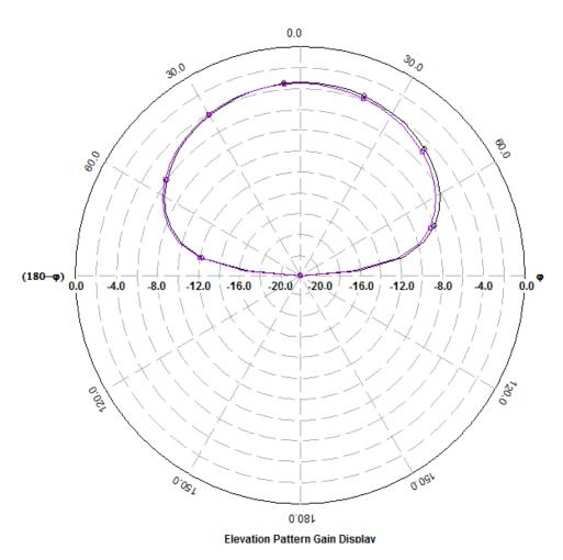
Fig. 3.9(a) Proposed antenna E- Plane pattern
