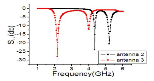
**Figure 2** Plot of  $S_{11}(dB)$  versus Frequency of the two antennas as illustrated in figure 1.
