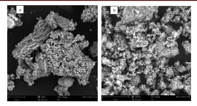
Figure 2. (a) Microstructure of Untreated POFA (b) Microstructure of Acidic Treatment
